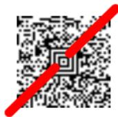
The aiming beam is smaller when the scanner is closer to the code and larger when it is farther from the code. Hold the scanner close to smaller bar codes, and farther away from large bar codes to get a proper read.
